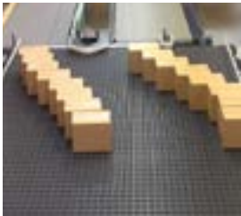
Activated Roller Belt (ARB) Sortation
